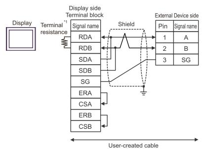
\*1 The resistance built into the Display is used as termination resistance. Please set the DIP Switch in the back of the Display as follows.
