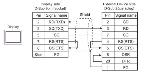
1B) Display side External Device side Terminal Block D-Sub 25pin (plug) Shield Pin Signal name Signal name RD(RXD) 2 SD Display SD(TXD) 3 RD SG 7 SG RS(RTS) 4 RS(RTS) CS(CTS) 5 CS(CTS) 6 **DSR** 20 DTR
