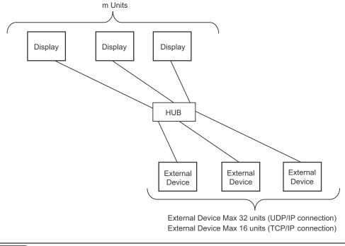
**NOTE** • The number of Display units has no limit. Note that more number of connecting units will result in increasing the communication load.
