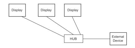
**NOTE** • The number of Display units has no limit. Note that more number of connecting units will result in increasing the communication load.
