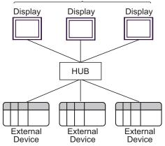
\* The maximum number of connectable units varies depending on the External Device. Refer to your External Device manual for details.
