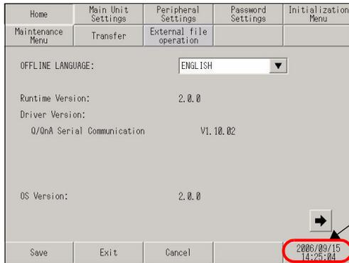
1. Enter offline mode, and touch the time display area in the control switches to display the [Time Setting] dialog box.
