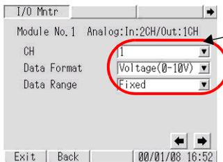
4. Touch each module No. After the corresponding screen appears, specify the I/O channel number, data format, and data range. (Example: CH “1”, Data Format “Voltage (0-10 V)”, Data Range “Fixed”)
