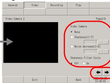
4. When the screen for [Video Display] opens, check the settings or touch the item that you want to change. To go to the next page, touch the right arrow key on the lower right of the screen.
