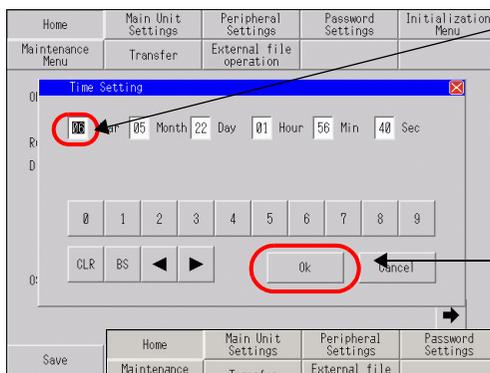
2. Touch the unit for the date or time to be changed. When the value is highlighted in black, enter a value using the numeric touch keys below.
