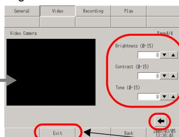
5. Touch [Exit], and when the [Exit] dialog box is displayed, touch [Save changes and exit]. The GP restarts automatically.
