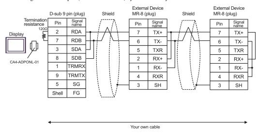
E) When using the terminal block conversion adapter (CA3-ADPTRM-01), the COM port conversion adapter (CA3-ADPCOM-01) by Pro-face and your own cable
