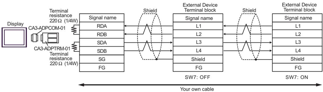
**NOTE** • When IPC is used as the Display, the terminal resistance of 220Ω can be inserted by the fact that the dip switch 5, 6 of IPC is turned to ON.
