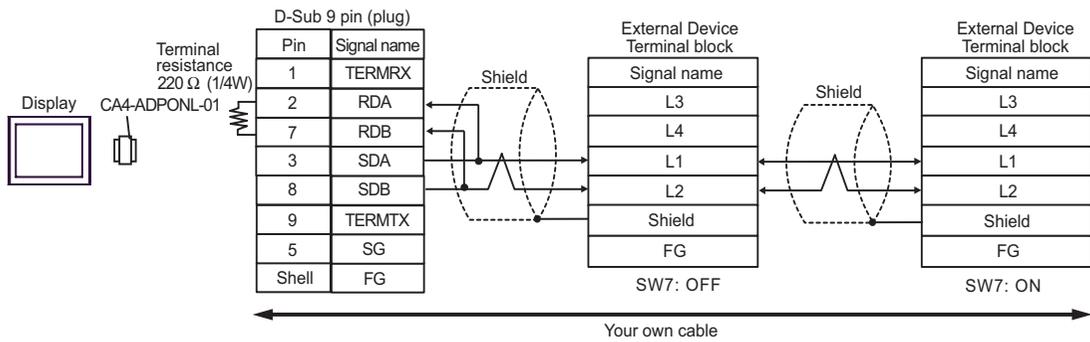
E. When using the COM port conversion adapter (CA3-ADPCOM-01), the terminal block conversion adapter (CA3-ADPTRM-01) by Pro-face and your own cable
