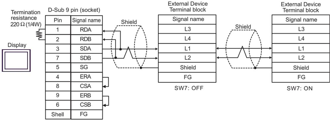
C. When using the online adapter (CA4-ADPONL-01), the terminal block conversion adapter (CA3-ADPTRM-01) by Pro-face and your own cable
