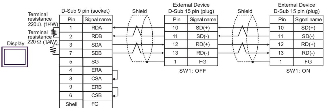
**NOTE** • When IPC is used as the Display, the terminal resistance of 220Ω can be inserted by the fact that the dip switch 5, 6 of IPC is turned to ON.
