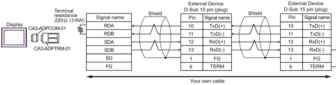
**NOTE** • When IPC is used as the Display, the terminal resistance of 220Ω can be inserted by the fact that the dip switch 6 of IPC is turned to ON.
