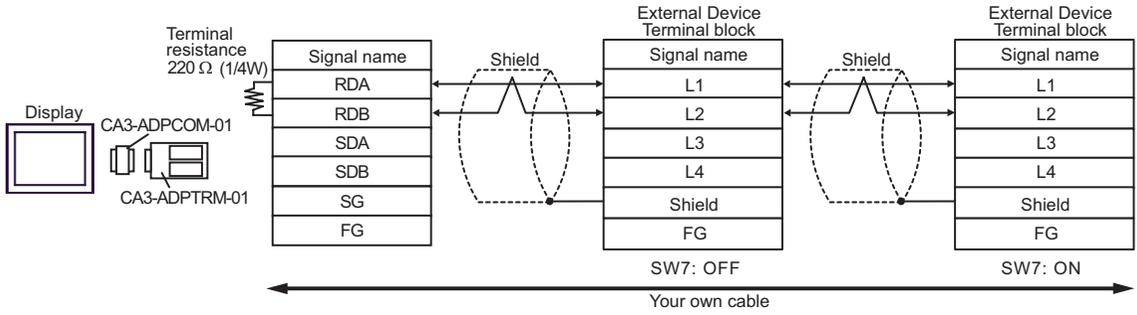
**NOTE** • When IPC is used as the Display, the terminal resistance of  $220\ \Omega$  can be inserted by the fact that the dip switch 6 of IPC is turned to ON.
