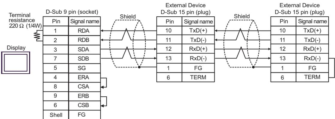
**NOTE** • When IPC is used as the Display, the terminal resistance of 220Ω can be inserted by the fact that the dip switch 6 of IPC is turned to ON.
