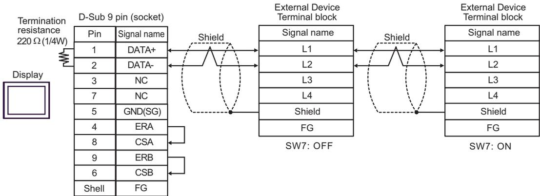
**NOTE** • When IPC is used as the Display, the terminal resistance of  $220\ \Omega$  can be inserted by the fact that the dip switch 6 of IPC is turned to ON.
