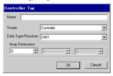
5) Input the Name, Data Type/Structure, and Array Dimensions, then click [OK].
