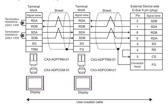
B) When using the COM port conversion adapter (CA3-ADPCOM-01), the multilink cable (CA3-CBLMLT-01) by Pro-face and user-created cable
