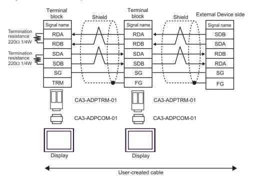
B) When using the COM port conversion adapter (CA3-ADPCOM-01), the multilink cable (CA3-CBLMLT-01) by Pro-face and user-created cable
