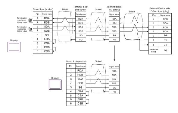
D) When using the online adapter (CA4-ADPONL-01), the connector terminal block conversion adapter (CA3-ADPTRM-01) by Pro-face and user-created cable
