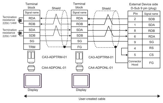
E) When using the online adapter (CA4-ADPONL-01), the multilink cable (CA3-CBLMLT-01) by Pro-face and user-created cable
