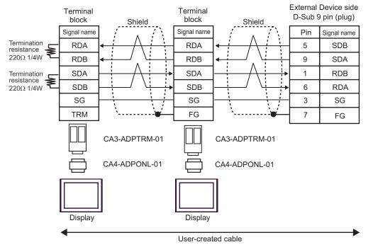
E) When using the online adapter (CA4-ADPONL-01), the multilink cable (CA3-CBLMLT-01) by Pro-face and user-created cable
