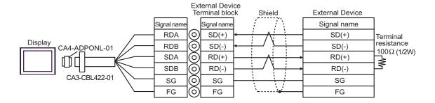
•  $100\Omega$  (1/2W) termination resistance is inserted between RDA and RDB in CA3-CBL422-01.
