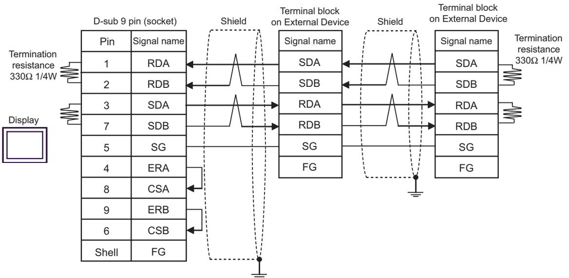
C) When using the online adapter (CA4-ADPONL-01), the connector terminal block conversion adapter (CA3-ADPTRM-01) by Pro-face and your own cable
