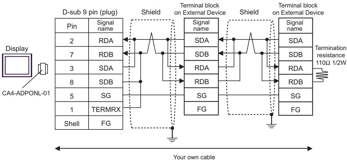
E) When using the COM port conversion adapter (CA3-ADPCOM-01), the connector terminal block conversion adapter (CA3-ADPTRM-01) by Pro-face and your own cable
