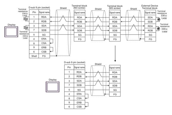
D) When using the online adapter (CA4-ADPONL-01), the connector terminal block conversion adapter (CA3-ADPTRM-01) by Pro-face and user-created cable
