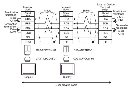
B) When using the COM port conversion adapter (CA3-ADPCOM-01), the multilink cable (CA3-CBLMLT-01) by Pro-face and user-created cable
