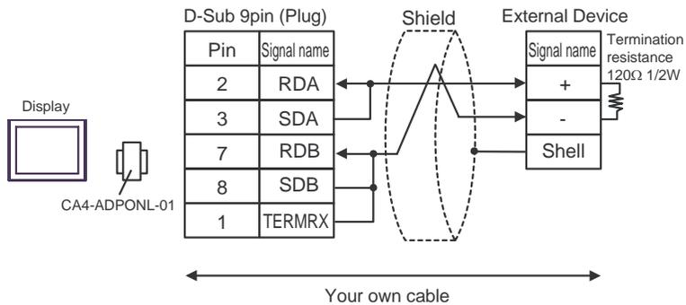
E) When using the COM port conversion adapter (CA3-ADPCOM-01), the connector terminal block conversion adapter (CA3-ADPTRM-01) by Pro-face and your own cable
