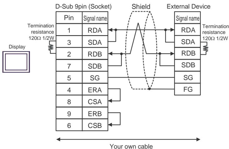
C) When using the online adapter (CA4-ADPONL-01), the terminal block conversion adapter (CA3-ADPTRM-01) by Pro-face and your own cable
