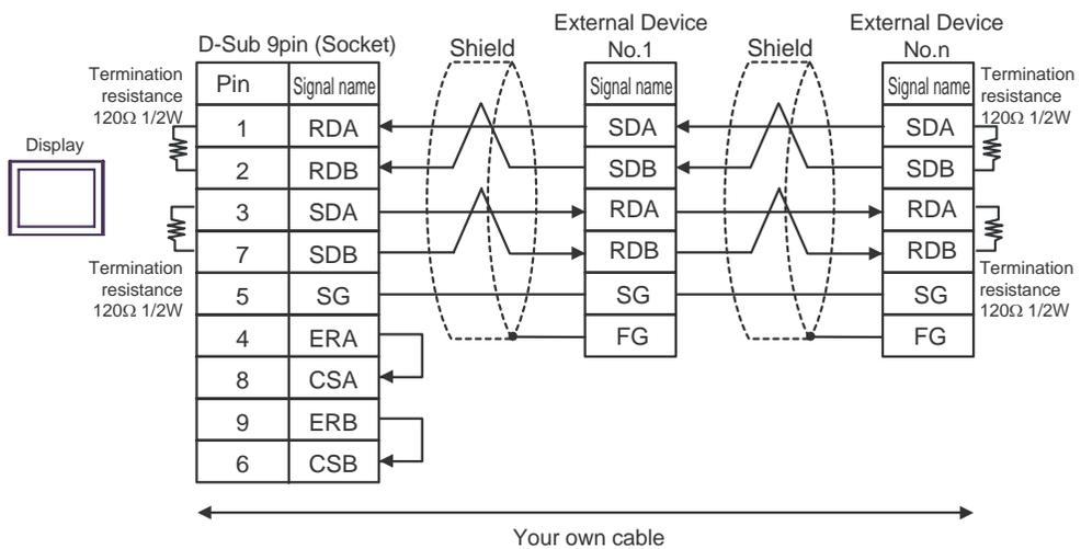
C) When using the online adapter (CA4-ADPONL-01), the terminal block conversion adapter (CA3-ADPTRM-01) by Pro-face and your own cable
