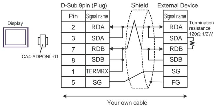
E) When using the COM port conversion adapter (CA3-ADPCOM-01), the terminal block conversion adapter (CA3-ADPTRM-01) by Pro-face and your own cable
