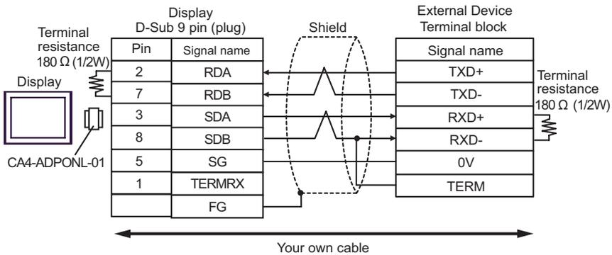
**NOTE** • Connect a 180Ω termination resistor to the +RXD and -RXD.
