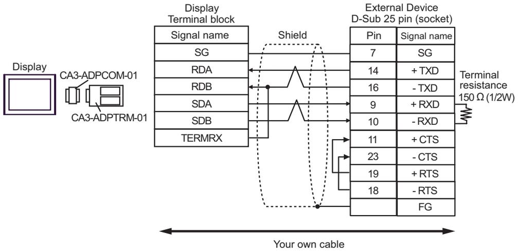
**NOTE** • Connect a 150Ω termination resistor to the +RXD and -RXD.
