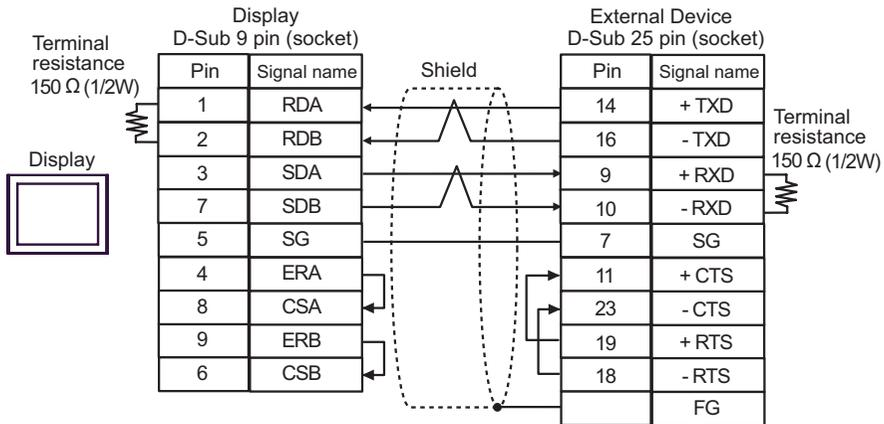
**NOTE** • Connect a 150Ω termination resistor to the +RXD and -RXD.
