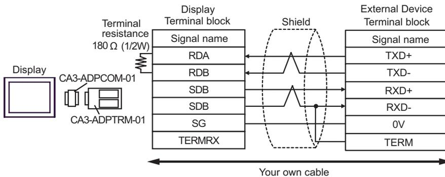
**NOTE** • Connect a 180Ω termination resistor to the +RXD and -RXD.
