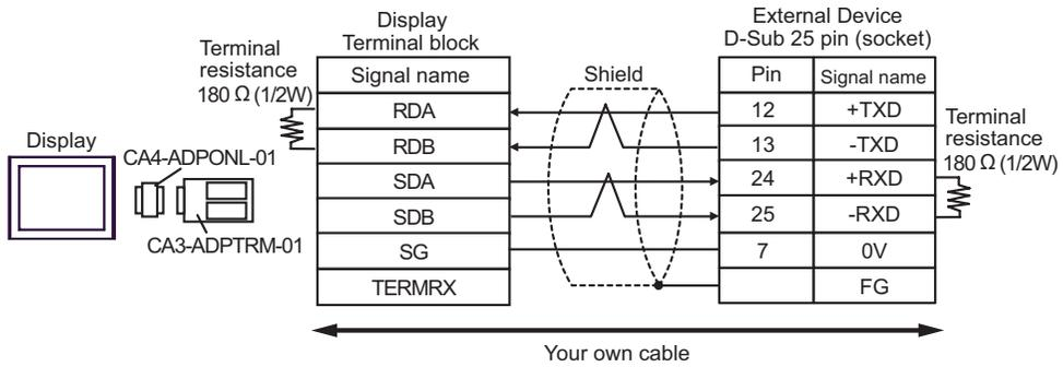
**NOTE** • Connect a 180Ω termination resistor to the +RXD and -RXD.
