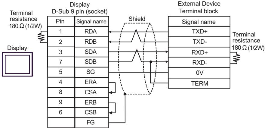
**NOTE** • Connect a 180Ω termination resistor to the +RXD and -RXD.
