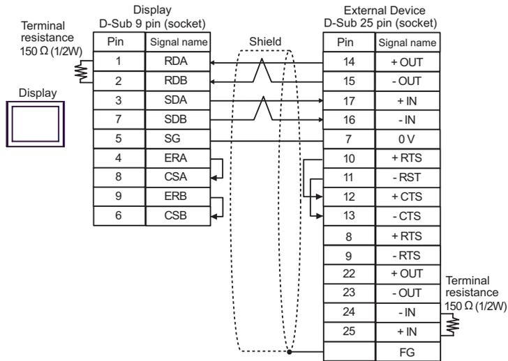
**NOTE** • Connect a 150Ω termination resistor to the +IN and -IN that are not used.
