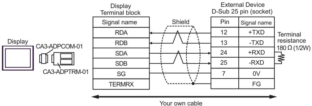
**NOTE** • Connect a 180Ω termination resistor to the +RXD and -RXD.
