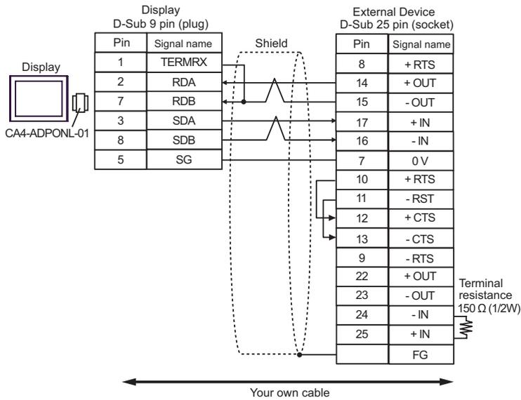
**NOTE** • Connect a 150Ω termination resistor to the +IN and -IN that are not used.
