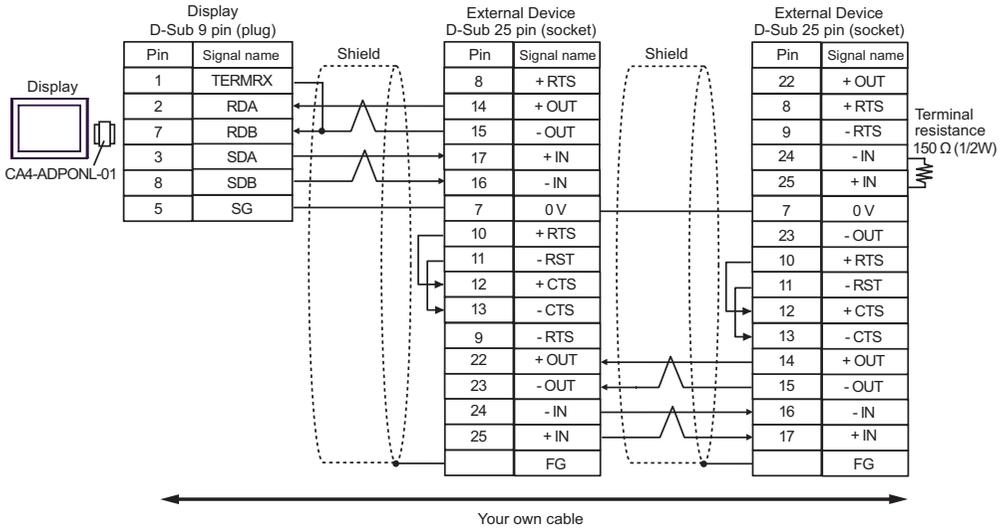
**NOTE** • Connect a 150Ω termination resistor to the +IN and -IN that are not used.
