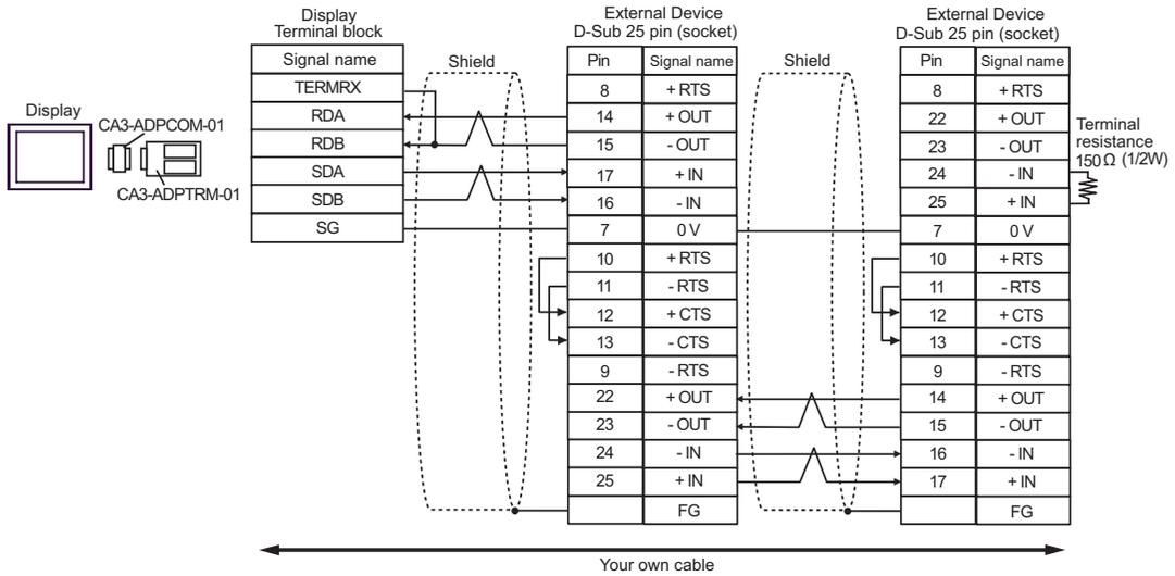
**NOTE** • Connect a 150Ω termination resistor to the +IN and -IN that are not used.
