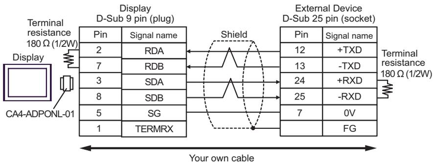
**NOTE** • Connect a 180Ω termination resistor to the +RXD and -RXD.
