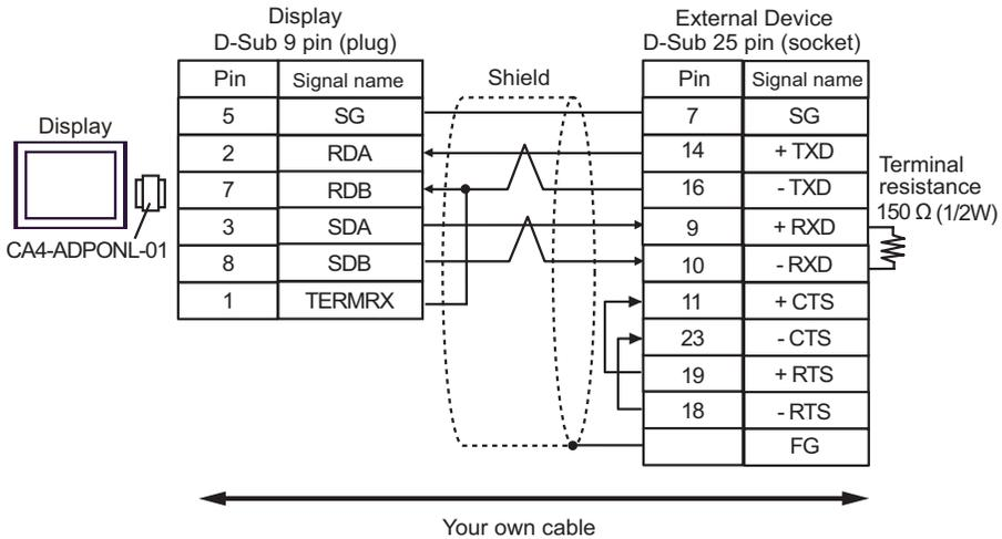
**NOTE** • Connect a 150Ω termination resistor to the +RXD and -RXD.
