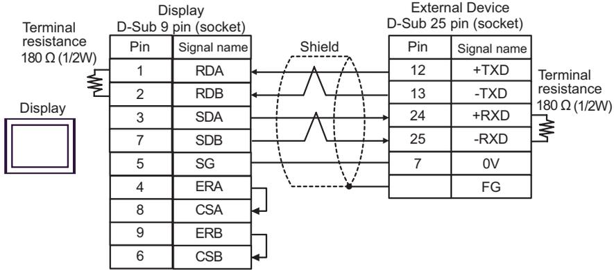
**NOTE** • Connect a 180Ω termination resistor to the +RXD and -RXD.
