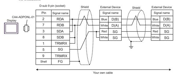
E) When using the COM port conversion adapter (CA3-ADPCOM-01), the connector terminal block conversion adapter (CA3-ADPTRM-01) by Pro-face and the accessory box (TSX SCA 50) by Schneider Electric
