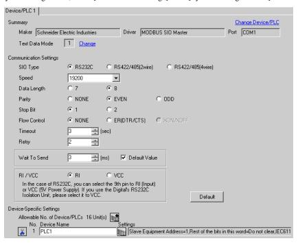
To display the setting screen, click [fig. ([Setting]) of External Device you want to set from [Device-Specific Settings] of [Device/PLC Settings].
