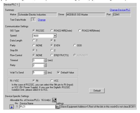
To display the setting screen, click [Market ([Setting]) of External Device you want to set from [Device-Specific Settings] of [Device/PLC Settings].
