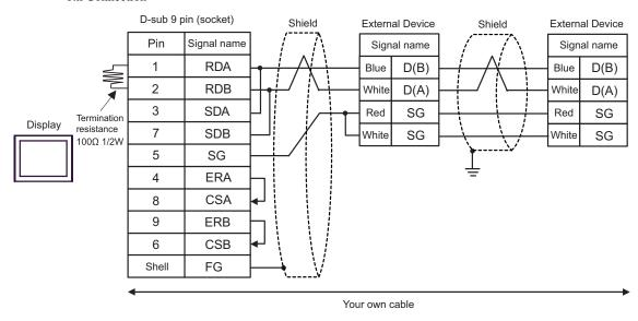
C) When using the online adapter (CA4-ADPONL-01), the connector terminal block conversion adapter (CA3-ADPTRM-01) by Pro-face, your own cable and the accessory box (TSX SCA 50) by Schneider Electric
