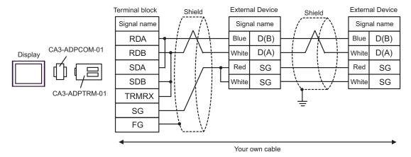
B) When using the accessory box (TSX SCA 50) by Schneider Electric and your own cable
