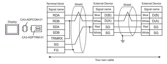
F) When using the accessory box (TSX SCA 50) by Schneider Electric and your own cable
