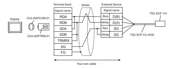
B) When using your own cable, the Uni-Telway connection cable (TSX SCP CU 4030) and the PCMCIA card for RS485 (TSX SCP 114) by Schneider Electric
