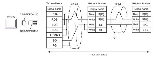
D) When using the online adapter (CA4-ADPONL-01) by Pro-face and the accessory box (TSX SCA 50) by Schneider Electric
