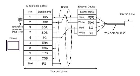
C) When using the online adapter (CA4-ADPONL-01), the connector terminal block conversion adapter (CA3-ADPTRM-01) by Pro-face, the Uni-Telway connection cable (TSX SCP CU 4030) and the PCMCIA card for RS485 (TSX SCP 114) by Schneider Electric
