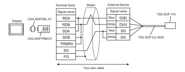
D) When using the online adapter (CA4-ADPONL-01) by Pro-face, your own cable, the Uni-Telway connection cable (TSX SCP CU 4030) and the PCMCIA card for RS485 (TSX SCP 114) by Schneider Electric
