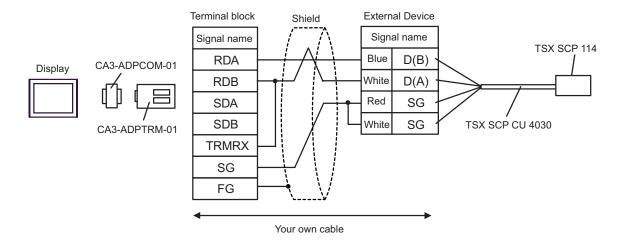
F) When using your own cable, the Uni-Telway connection cable (TSX SCP CU 4030) and the PCMCIA card for RS485 (TSX SCP 114) by Schneider Electric
