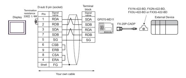
C) When using the online adapter (CA4-ADPONL-01) by Pro-face, the 2-port adapter cable for AGP (CA3-MDCB11) by Pro-face, the 2-port adapter II (GP070-MD11) by Pro-face, the connector conversion cable (FX-20P-CADP) by Mitsubishi Electric Corp. and the function extension board (FX1N-422-BD, FX2N-422-BD, FX3U-422-BD or FX3G-422-BD) by Mitsubishi Electric Corp.
