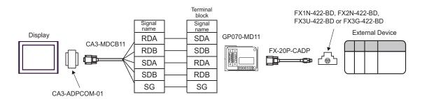
B) When using your own cable, the 2-port adapter II (GP070-MD11) by Pro-face, the connector conversion cable (FX-20P-CADP) by Mitsubishi Electric Corp., and the function extension board (FX1N-422-BD, FX2N-422-BD, FX3U-422-BD or FX3G-422-BD) by Mitsubishi Electric Corp.
