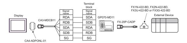
D) When using the online adapter (CA4-ADPONL-01) by Pro-face, your own cable, the 2-port adapter II (GP070-MD11) by Pro-face, the connector conversion cable (FX-20P-CADP) by Mitsubishi Electric Corp. and the function extension board (FX1N-422-BD, FX2N-422-BD, FX3U-422-BD or FX3G-422-BD) by Mitsubishi Electric Corp.
