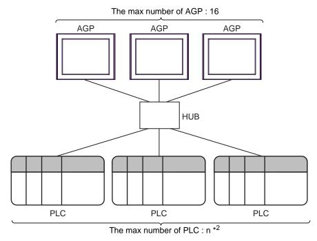
\*2 The maximum 32 PLCs connection by UDP connection, the maximum 16 PLCs connection by TCP connection.
