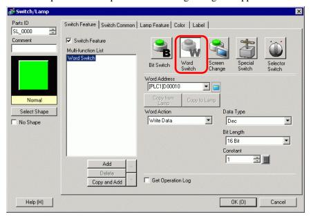
4 Set the address (D102) where you want to write data when you touch the switch in [Word Address].
