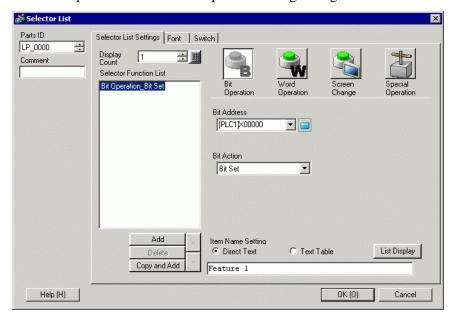
3 Create the switch to operate the bit.
