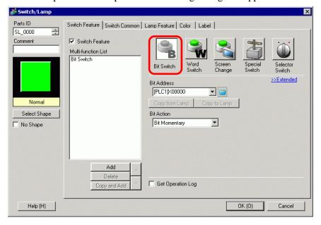
Click the icon to display Select device "M", input an address input keypad. "100" as the address, and press the "Ent" key. 💰 Input Address Bit Address Bit Address Device/PLC PLC1 [PLC1]X00000 [PLC1]M000100 ▼ 100 М Back Clr Click A 8 В C 9 D E F 5 6 2 3 0 Ent ✓ Set as Default Value
