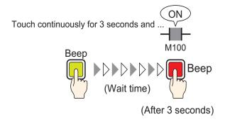
If the Switch is pressed continuously for a set time (for example, 3 seconds), the specified bit will turn ON. This is useful in preventing accidental input.
