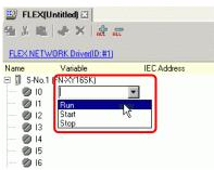
**3** Press the [Enter] key to map the address and display the I/O address (IEC Address).
