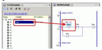
2 The address will be mapped and the I/O address (IEC address) will be displayed.
