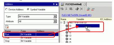
4 The address will be mapped and the I/O address (IEC address) will be displayed.
