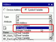
3 The list displays addresses whose [Type] equals [Bit Variable]. In the list, drag "Start" to the instruction operand you want to map the variable. Release the mouse when the pointer changes from  $\bigcirc$  to  $\triangleright$ <sub>ta</sub>.
