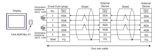
• In order to improve noise resistance characteristics, please use a twist pair whole shield cable as a transmission cable and ground the shield line.
