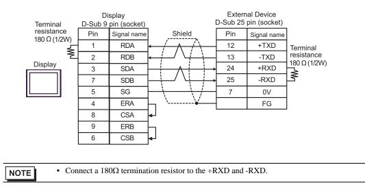
C.When using the online adapter (CA4-ADPONL-01), the connector terminal block conversion adapter (CA3-ADPTRM-01) by Digital Electronics Corp., and your own cable
