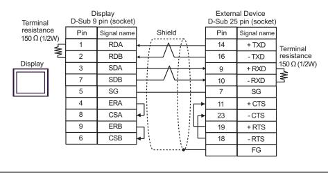
• Connect a  $150\Omega$  termination resistor to the +RXD and -RXD.
