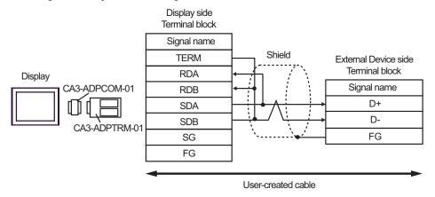
The following is a cable diagram for connecting the GP3000H series using the abovementioned External Device connection cable:
