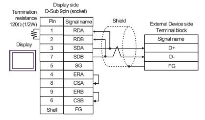
The following is a cable diagram for connecting the GP3000H series using the abovementioned External Device connection cable:
