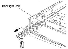
(9) Insert a new Backlight Unit while sliding it along the groove.
