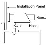
The following shows the insertion slots location that are on both left and right sides. (GP-3200 Series)
