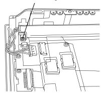
(7) Lift the edge of the Backlight Unit, and remove the unit while sliding it along the groove
