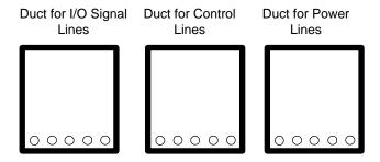
If different wires must be placed in the same duct, separate them with an earthed/grounded divider.
