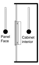
Be sure that heat from surrounding equipment does not cause the GP to exceed its standard operating temperature. • When installing the GP in a slanted panel, the panel face should not incline more than 30°.
