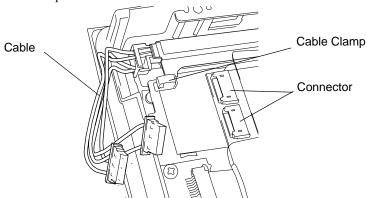
(7) Remove the hook from the Backlight Unit.
