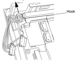
(8) Remove the Backlight Unit while sliding it along the groove.
