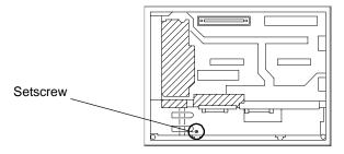
(5) Open the circuit board chassis, it's turn left to right.
