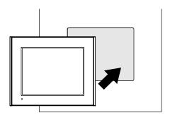
(2) Insert the installation fasteners into the GP insertion slots, at the left-and-right or topand-bottom of the unit. (total: 4 slots). Only the AGP-3750T has 8 slot locations.
