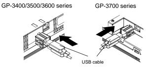
(4) Attach the USB cover to fix the USB cable. Insert the USB cover into the tab of the USB Holder.
