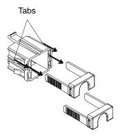
(2) Attach the USB Holder to the USB Host Interface part of the main unit. Hook the upper pick of the USB holder to the attachment hole of the main unit and then insert the lower pick as shown below to fix the USB holder.
