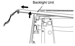
(8) Insert a new Backlight Unit while sliding it along the groove.
