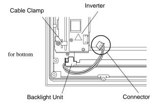
(7) As shown here, push the backlight unit's attachment clip to the right to release the backlight unit.
