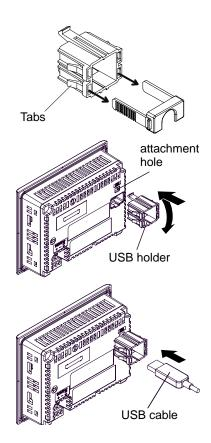
(4) Attach the USB cover to fix the USB cable. Insert the USB cover into the tab of the USB Holder.
