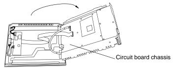
A hot circuit board chassis can burn you. Be sure the chassis has cooled completely prior to replacing the backlights.
