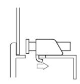
(4) Use a Phillips screwdriver to tighten each fastener screw and secure the GP in place.
