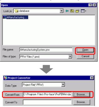
4 In [Convert-To], designate a GP-Pro EX project file (\*.prx). Click the [Browse] button, input a new [File name] (For example "AManufacturingSystem.prx"), and click \_\_\_\_\_\_\_. A new project file name is set to [Convert-To].
