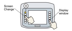
You can set up often-used switch and key features on the Hand-held GP's local function keys, which operate only when the associated screen is displayed.
