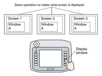
You can set up global function keys on the Hand-held GP so they can be used on all screens.
