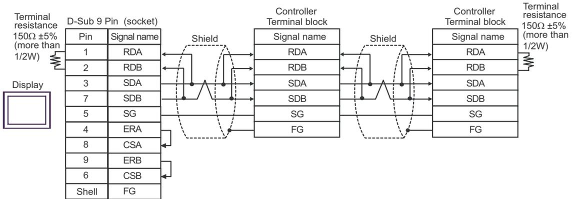
C. When using the online adapter (CA4-ADPONL-01), the connector terminal block conversion adapter (CA3-ADPTRM-01) by Pro-face, and your own cable
