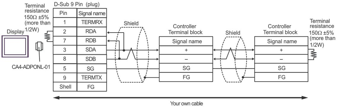
E. When using the COM port conversion adapter (CA3-ADPCOM-01), the connector terminal block conversion adapter (CA3-ADPTRM-01) by Pro-face, and your own cable
