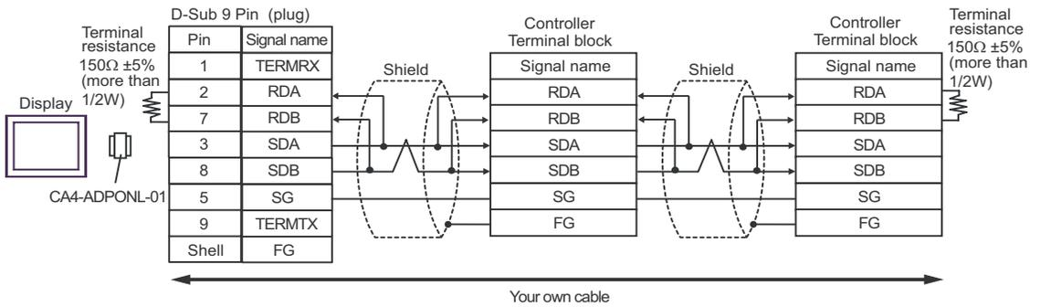
E. When using the COM port conversion adapter (CA3-ADPCOM-01), the connector terminal block conversion adapter (CA3-ADPTRM-01) by Pro-face, and your own cable
