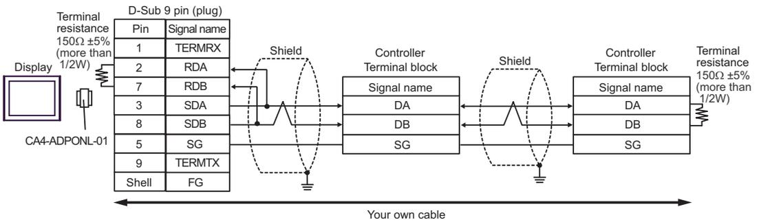
E. When using the COM port conversion adapter (CA3-ADPCOM-01), the connector terminal block conversion adapter (CA3-ADPTRM-01) by Pro-face, and your own cable
