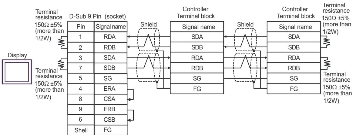
C. When using the online adapter (CA4-ADPONL-01), the connector terminal block conversion adapter (CA3-ADPTRM-01) by Pro-face, and your own cable
