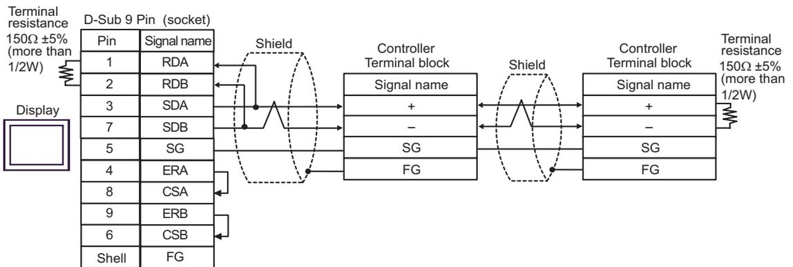
C. When using the online adapter (CA4-ADPONL-01), the connector terminal block conversion adapter (CA3-ADPTRM-01) by Pro-face, and your own cable
