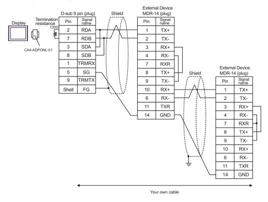
E) When using the COM port conversion adapter (CA3-ADPCOM-01), the terminal block conversion adapter (CA3-ADPTRM-01) by Pro-face and your own cable
