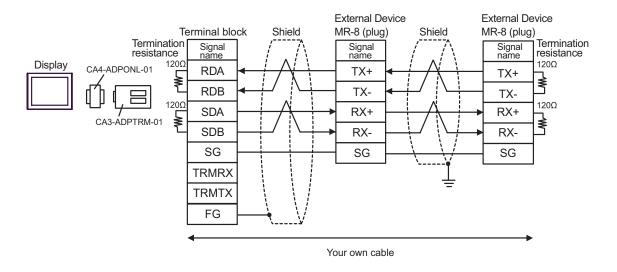
NOTE • When the External device has the SG terminal, connect it to the SG terminal of the Display.
