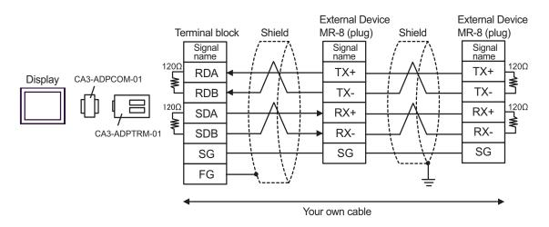
**NOTE** • When the External device has the SG terminal, connect it to the SG terminal of the Display.
