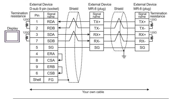
• When the External device has the SG terminal, connect it to the SG terminal of the Display.
