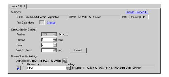
To display the setting screen, click [fig. ([Setting]) of External Device you want to set from [Device-Specific Settings] of [Device/PLC Settings].
