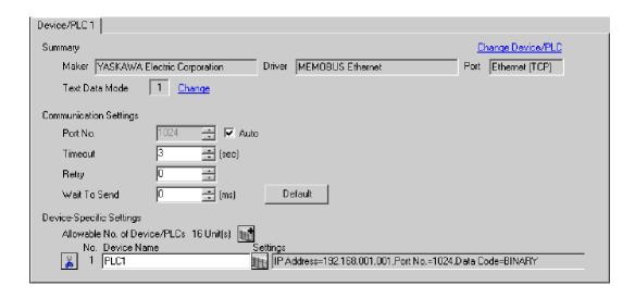
To display the setting screen, click [fig. ([Setting]) of External Device you want to set from [Device-Specific Settings] of [Device/PLC Settings].
