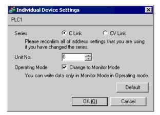
Set the HOST link unit attached to the External Device as below.
