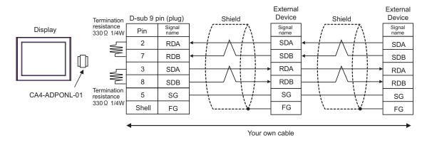
• In order to improve noise resistance characteristics, please use a twist pair whole shield cable as a transmission cable and ground the shield line.
