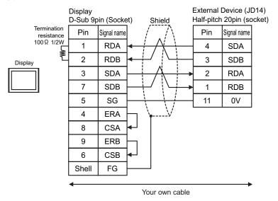
C) When using the online adapter (CA4-ADPONL-01), the terminal block conversion adapter (CA3-ADPTRM-01) by Pro-face and your own cable
