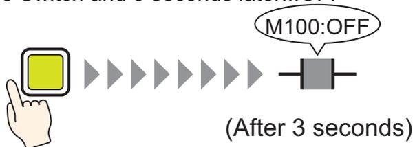
After the Switch is pressed and released, the specified bit will wait a set amount of time (for example, 3 seconds) before turning OFF.
