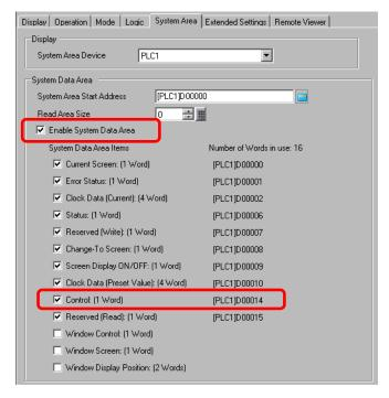
4 If you turn ON Bit 1 in the [Control: (1 Word)] address specified in step 3 while Bit 4 is OFF, the GP display unit buzzer rings.
