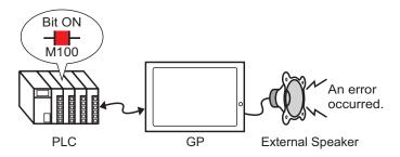
If you connect a GP sound output to an alarm, the GP can announce errors with sound. Sound output requires an external speaker (sold separately).
