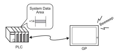
You can sound the GP internal buzzer from a device/PLC. You need to set the GP system data area in the PLC to sound the buzzer.
