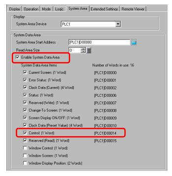
4 If you turn ON Bit 1 in the [Control: (1 Word)] address specified in step 3 while Bit 5 is OFF, the contact to sound an external buzzer turns ON. You can then connect and operate an external power supply and a buzzer or revolving light.
