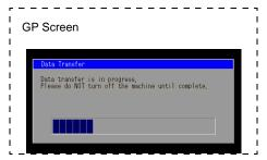
7 When the transfer finishes, the status changes from [Transferring] to [Transfer Complete]. Click [Close].
