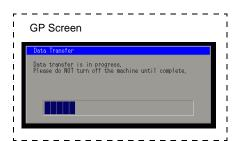
7 When the transfer finishes, the status changes from [Transferring] to [Transfer Complete]. Click [Close]. The GP is reset and the transferred screens are displayed.
