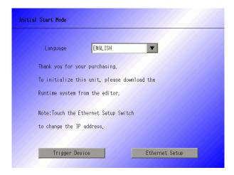
4 On the GP-Pro EX state tool bar, click the Transfer Project icon Transfer Project. The [Transfer Tool] dialog appears.
