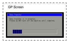
8 When the transfer finishes, the status changes from [Transferring] to [Transfer Complete]. Click [Close]. The GP is reset and the transferred screens are displayed.
