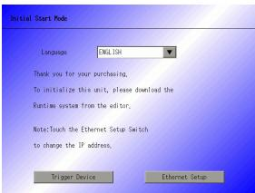
This screen will appear when you first connect the GP's power cord. After transferring a project once, this screen will not appear.
