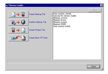
8 Copy or move all data created in the CF Card folder to the CF Card. The data, project backup data, and the CF Card Memory Loader Tool are all transferred to the CF Card.
