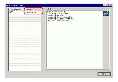
5 When the transfer finishes, the status changes from [Transferring] to [Transfer Complete]. Click [Close].
