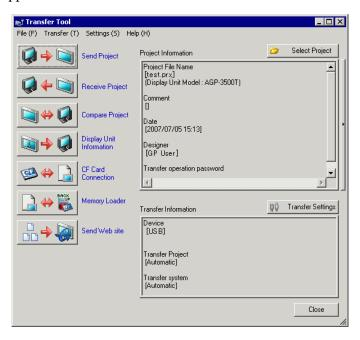
3 In [Transfer Information], acknowledge that [Device] is [USB]. If [USB] is not selected, click [Transfer settings] to display the [Transfer settings] dialog box below. In [Communication Port Settings], select [USB] and click [OK].
