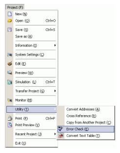
During the Error Check, the following dialog box appears. This dialog box closes when the Error Check is finished.
