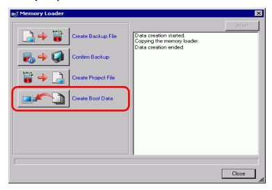
4 Move or copy all the created data to the CF Card/USB storage. The CF Card/USB storage device is now ready.
