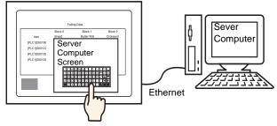
the display unit, you can operate the server computer screen if you connect the mouse and keypad registration to the USB port of the unit.
