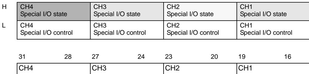
If the start bit of the CH (0 bit) is 1, the output is ON. If it is 0, the output is OFF.
