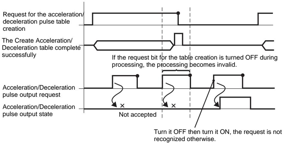
■ **Output State Status and Output Completed Status of Accelerating Pulse Output**
