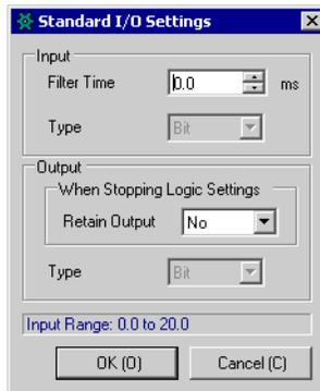
**NOTE** • When CH1 to CH4 are all set to "Standard", [Type] can be set to "Bit" or "Word".
