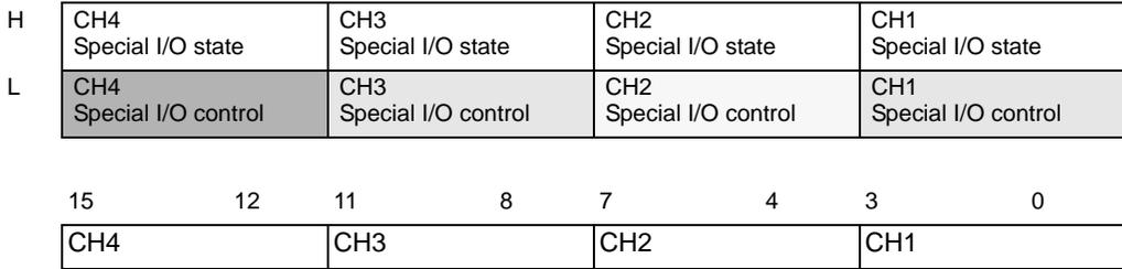
Turn ON the start bit of the CH (0 bit) to start and turn it OFF to stop the output.
