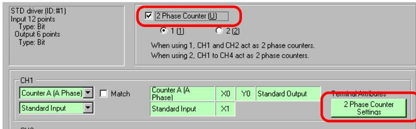
3 The [2 Phase Counter Settings] dialog box appears. Select the phase calculation mode from the pull-down menu.
