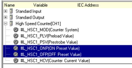
2 To specify the value from the system variable, change the parameter under [Request Special I/O Parameter Change].
