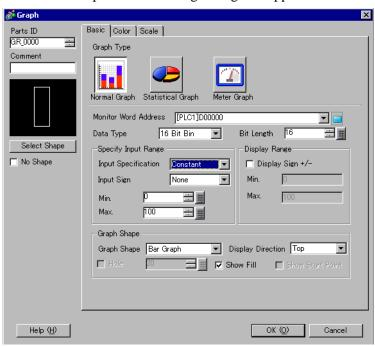
3 In [Monitor Word Address], set the address you want to display. Then set the [Data Type] and [Bit Length].
