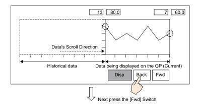
Touching the "Fwd" switch scrolls the data forwards the recent data samples by the predetermined scroll number.
