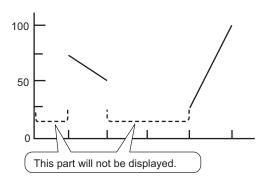
• If the [Data Type] of the historical trend graph part is set to [BCD] and the sampled data that includes A to Fh except BCD (except 0 to 9) is stored, the graph containing the previous sampled data will be displayed.<
