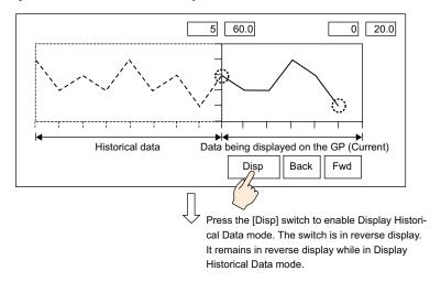
Touching the "Back" switch scrolls the data backward by the predetermined scroll number and displays previous data records.
