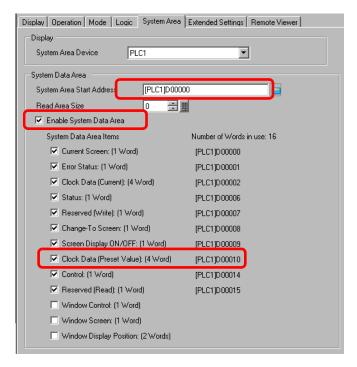
4 Write clock data to the address displayed in [Clock Data (Setting Value):(4 Words)] with BCD. Clock data is rewritten if the data rewrite flag changes from OFF → ON or ON → OFF. The procedure for writing data is as follows.
