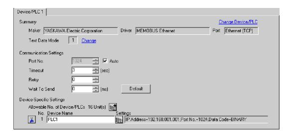
To display the setting screen, click [Mark ([Setting]) of External Device you want to set from [Device-Specific Settings] of [Device/PLC Settings].
