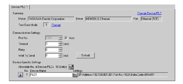
To display the setting screen, click [Mark ([Setting]) of External Device you want to set from [Device-Specific Settings] of [Device/PLC Settings].
