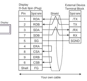
C) When using the online adapter (CA4-ADPONL-01), the terminal block conversion adapter (CA3-ADPTRM-01) by Pro-face and your own cable
