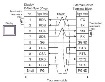
C) When using the online adapter (CA4-ADPONL-01), the terminal block conversion adapter (CA3-ADPTRM-01) by Pro-face and your own cable
