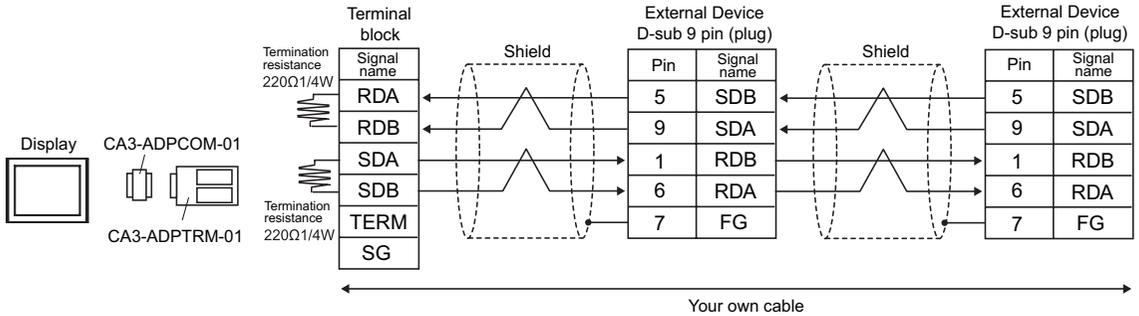
**NOTE** • When the display unit you use is an IPC, turn ON the DIP switches 5 and 6 to insert the termination resistance.
