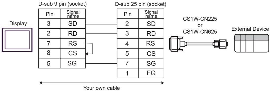
B) When using CS1W-CN226 (2m) or CS1W-CN626 (6m) by OMRON Corporation or your own cable
