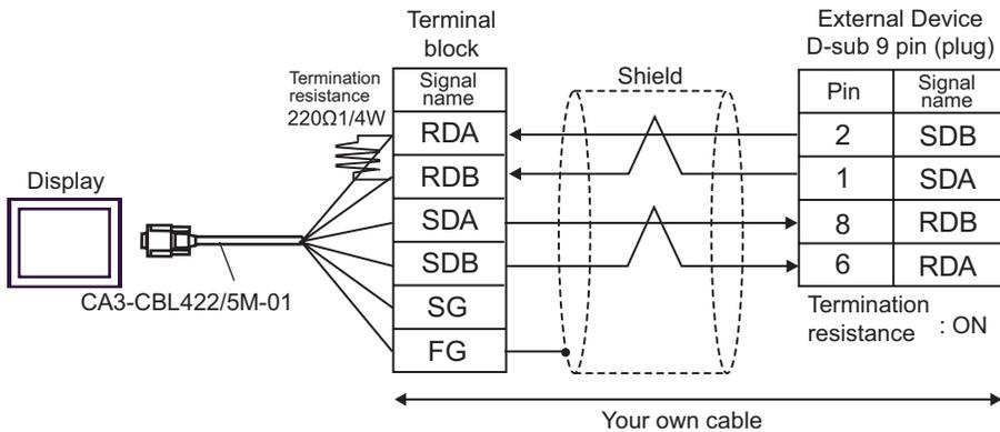
D) When using the online adapter (CA4-ADPONL-01), the terminal block conversion adapter (CA3-ADPTRM-01) by Pro-face and your own cable
