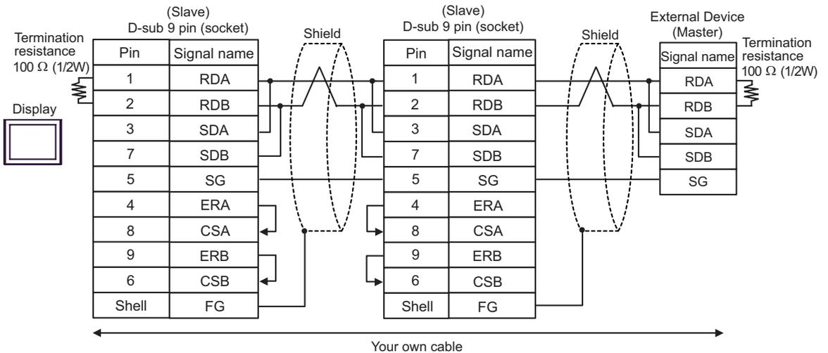
C. When using the online adapter (CA4-ADPONL-01), the terminal block conversion adapter (CA3-ADPTRM-01) by Pro-face and your own cable
