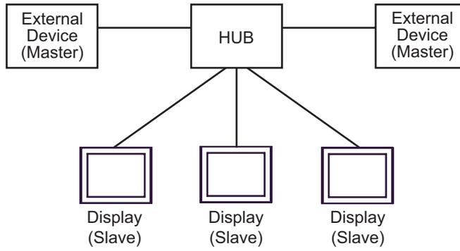
You can connect maximum 16 units of External Device (Master). Note that there is no communication between the Displays (Slaves).
