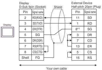
\*1 When connecting with 30i-Model A, 31i-Model A or 32i-Model A, The pin number of SG changes with ports to be used.
