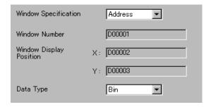
5 Click [OK]. The Window is configured according to the value stored in the address.
