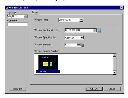
3 In [Window Control Address], set the word address (D100) that controls the window.
