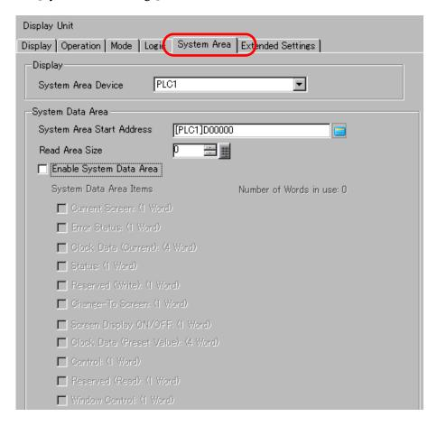
5 In [System Area Device], select the appropriate device that uses the system area. In [System Area Start Address], define the top address.
