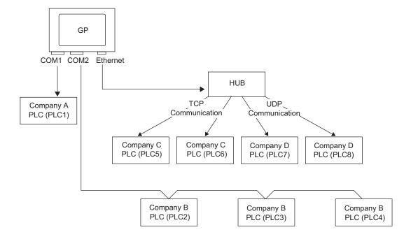
Multiple devices/PLCs can be connected simultaneously to one GP using four drivers (COM1, COM2, and Ethernet (UDP/TCP)).
