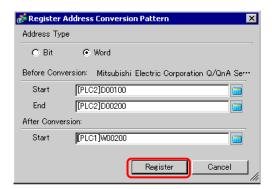
8 When the [Address Conversion Method Specification] dialog box appears and the conversion pattern is added, click [Convert].
