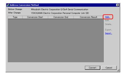
6 When the [Register Address Conversion Pattern] dialog box appears, set the [Address Type], the Before Conversion [Start] and [End] address, and the After Conversion [Start] address.
