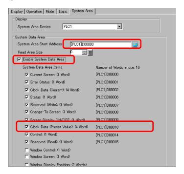
**4** Write "FFFFh" to the address displayed in [Screen Display ON/OFF: (1 Word)]. The GP screen display turns OFF.
