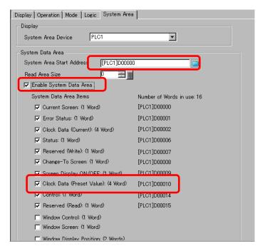
4 Write clock data to the address displayed in [Clock Data (Setting Value):(4 Words)] with BCD. Clock data is rewritten if the data rewrite flag changes from OFF → ON or ON → OFF. The procedure for writing data is as follows.
