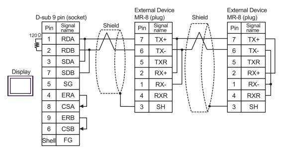
C) When using the online adapter (CA4-ADPONL-01), the terminal block conversion adapter (CA3-ADPTRM-01) by Pro-face and your own cable
