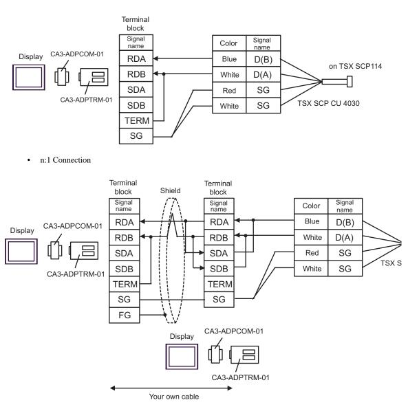
F) When using your own cable and Uni-Telway connection cable (TSX SCP CU 4030) by Schneider Electric Industries
