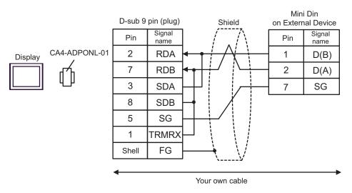
E) When using the COM port conversion adapter (CA3-ADPCOM-01), the connector terminal block conversion adapter (CA3-ADPTRM-01) by Pro-face and your own cable
