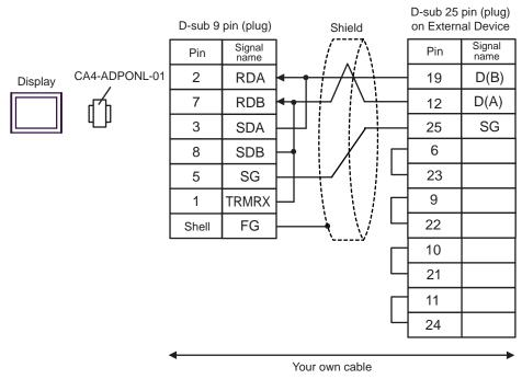
E) When using the COM port conversion adapter (CA3-ADPCOM-01), the connector terminal block conversion adapter (CA3-ADPTRM-01) by Pro-face and your own cable
