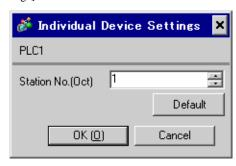
Use the rotary switch on Link I/F for setting. Please refer to the manual of the External Device for more details. Restart the power of the External Device after setting the switch to enable the setting.
