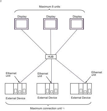
\*1 You can connect up to 32 units of External Device for UDP, and 16 units of External Device for TCP at the same time.
